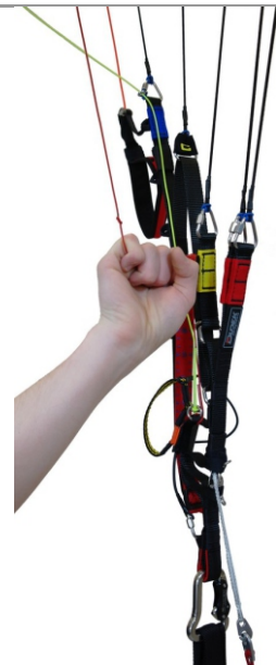
4 Steering with TEA line (trimmers partially or full released - accelerated mode).
