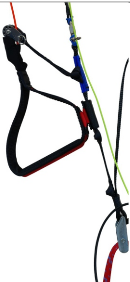
1 Pulley in first position (upper lengthened), EK magnet mounted over second pulley position.
