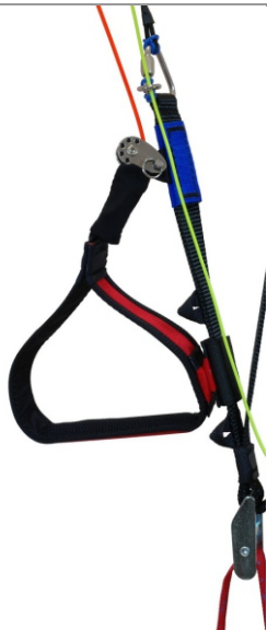
2 Pulley in first position, EK magnet mounted over buckle of the trimmer.
