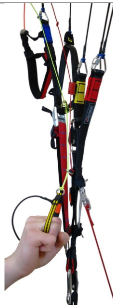
3 Steering with the TST only (trimmers partially or full released - accelerated mode)
