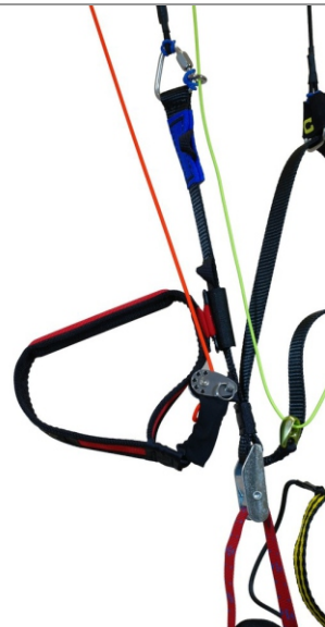
4 Pulley in third position (lower), EK magnet mounted over buckle of the trimmer.
