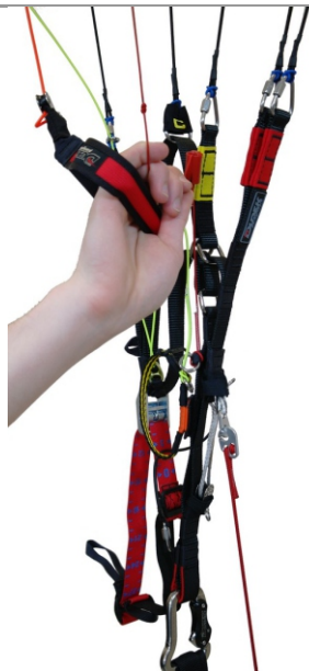
2 Brake handle + TEA line (trimmer partially released - accelerated mode)
