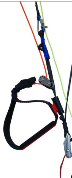
3 Pulley in second position (middle), EK magnet mounted over buckle of the trimmer.
