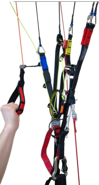
1 Steering with just the brake handle (trimmers colsed - slow mode)
