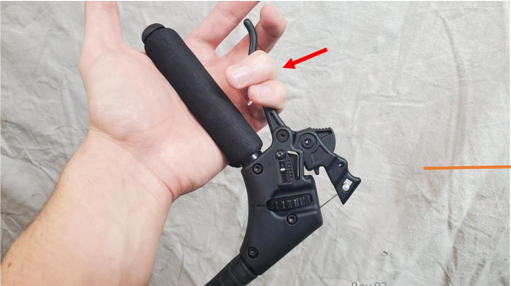
The throttle lock will snap out of position, disengaging the cruise control and bringing the pilot back in manual control.
