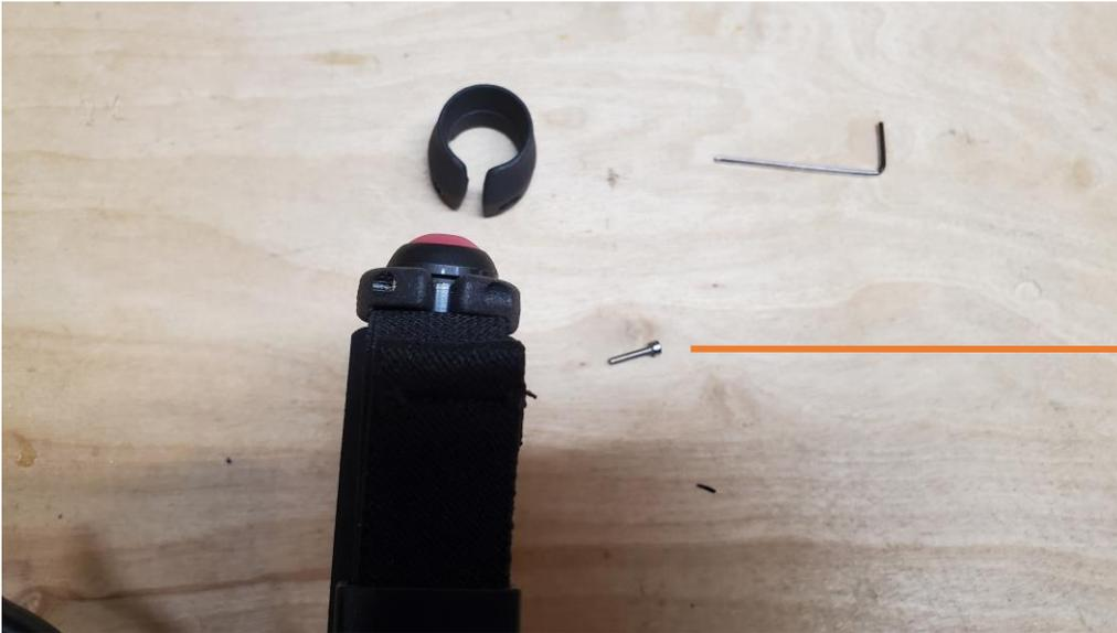
Completely remove the screw from the upper grip lock
