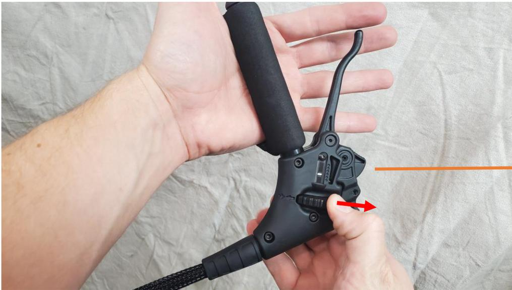
Turn the catch adjustment wheel as shown to move the catch downward.
