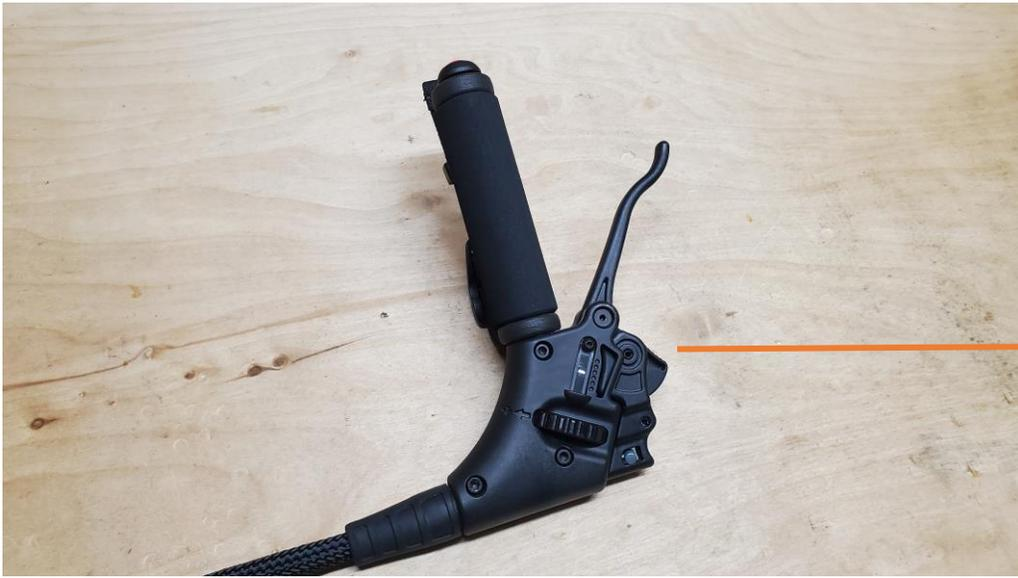
Out of the box, the grip screws will be loosely fitted to the handle to make it easy to setup for left or right handed use.
