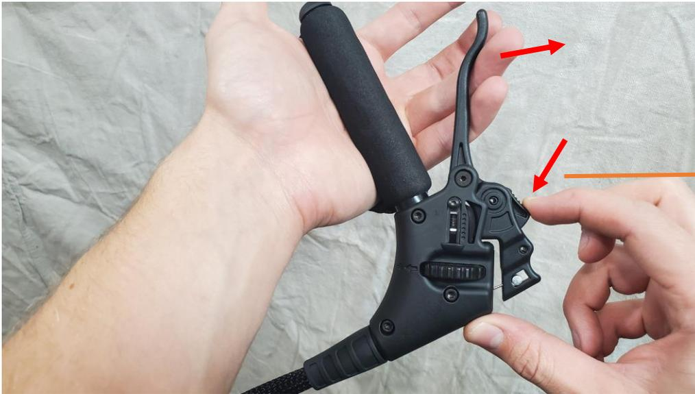
When the lock engages the internal catch, slowly let go of the throttle lever as shown.
