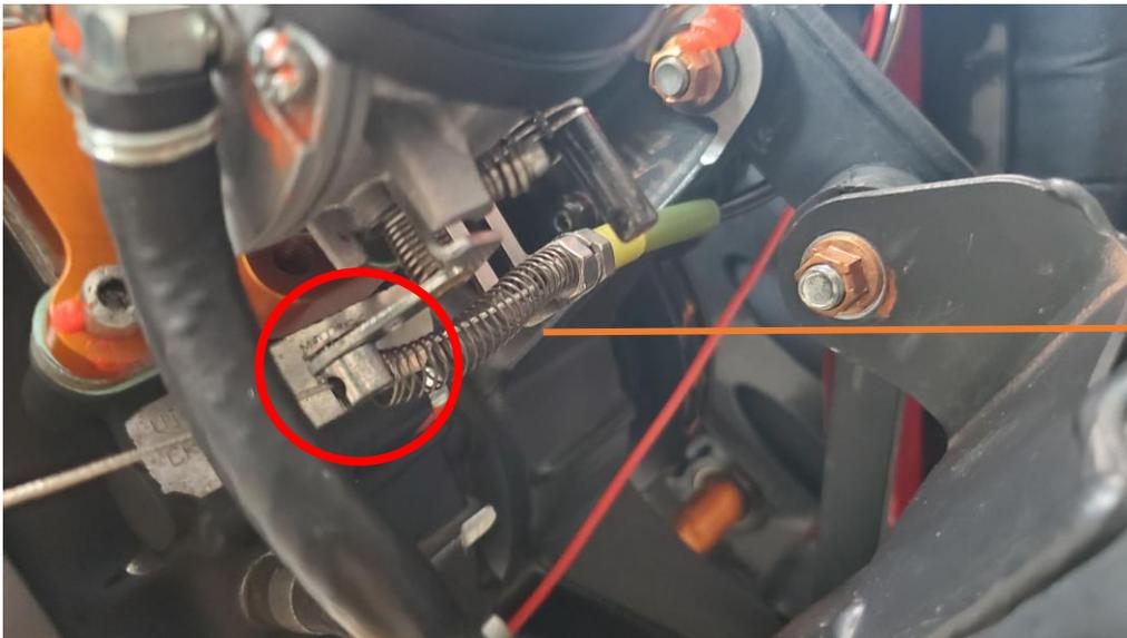
Place the cable through the slot as shown.
