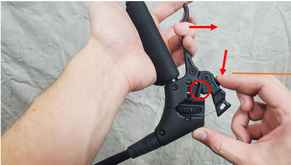
Keeping pressure on the throttle lock, slowly release pressure on the throttle lever. You will feel the lock engaging the catch internally.
