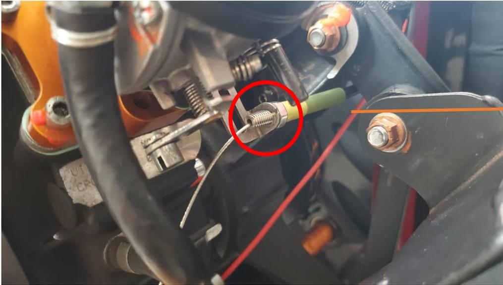
Slide barrel into position as shown.
