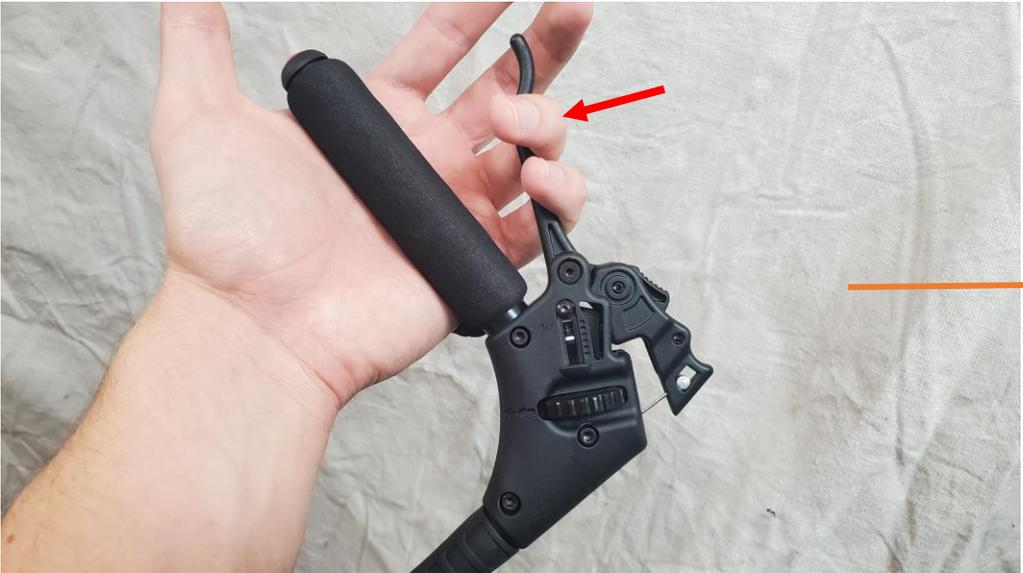
To disengage the cruise control, slightly pull the throttle lever inward as shown.
