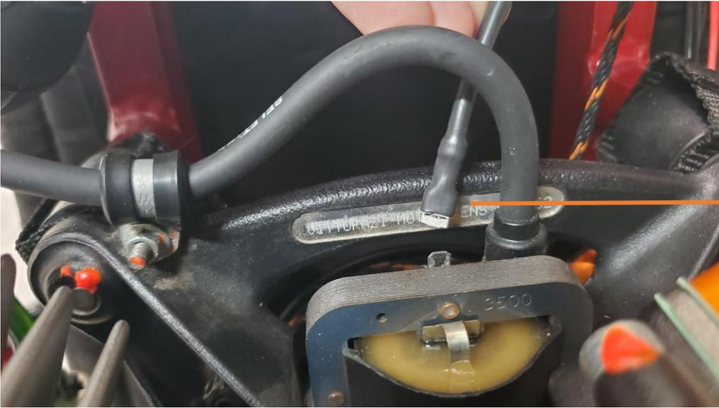
Feed the kill switch connector through the motor as desired
