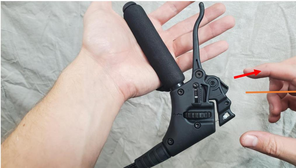
The mechanism is now in the locked position and does not require input from the pilot to maintain the engine RPM.
