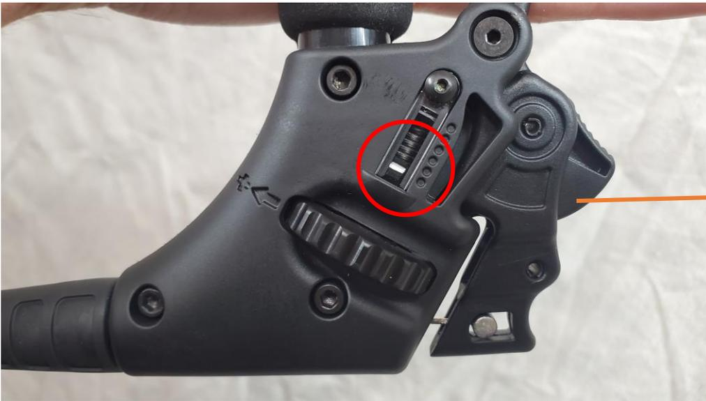
Note: The cruise control mechanism can be completely ignored by adjusting the internal catch to the bottom of the window. This will move the catch too low to possibly engage with the throttle lock.
