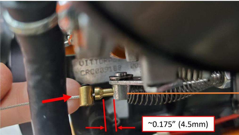
Slide the locking barrel over the cable and push against the sleeve.
