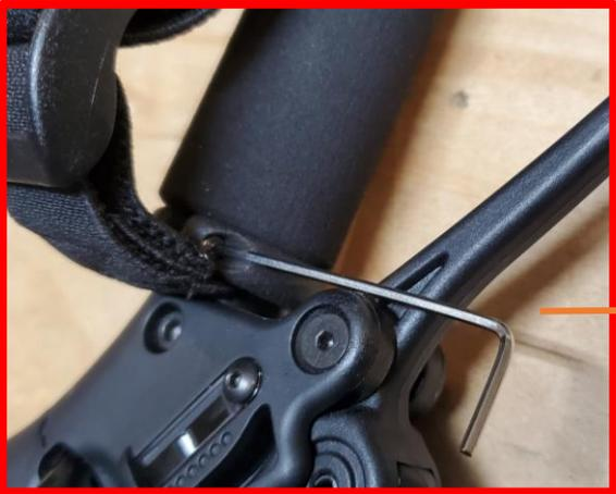
Use the included allen key to unscrew the top and bottom grip screws
