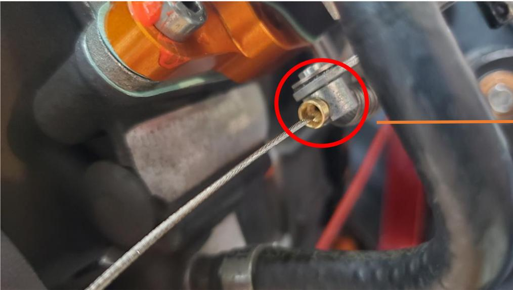
Push the sleeve into the hole as shown.
