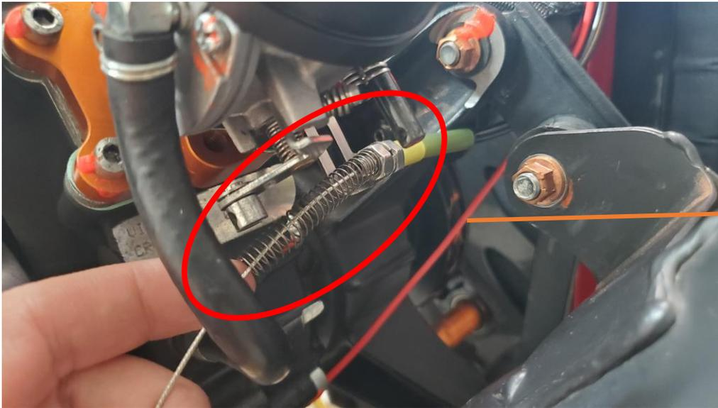
Slide the spring over the cable and push up against the barrel.
