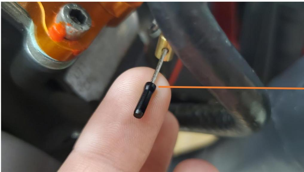
Slide the cap over the cable end
