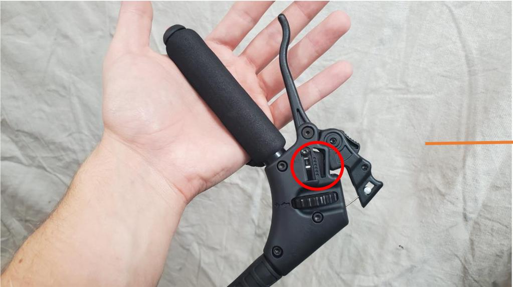
When the desired engine RPM is reached, the system will remain locked in this position until the throttle lever is reengaged.
