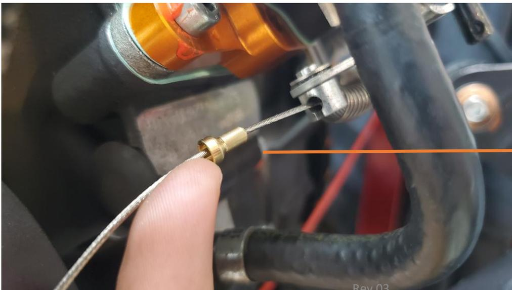
Slide the sleeve over the cable as shown.
