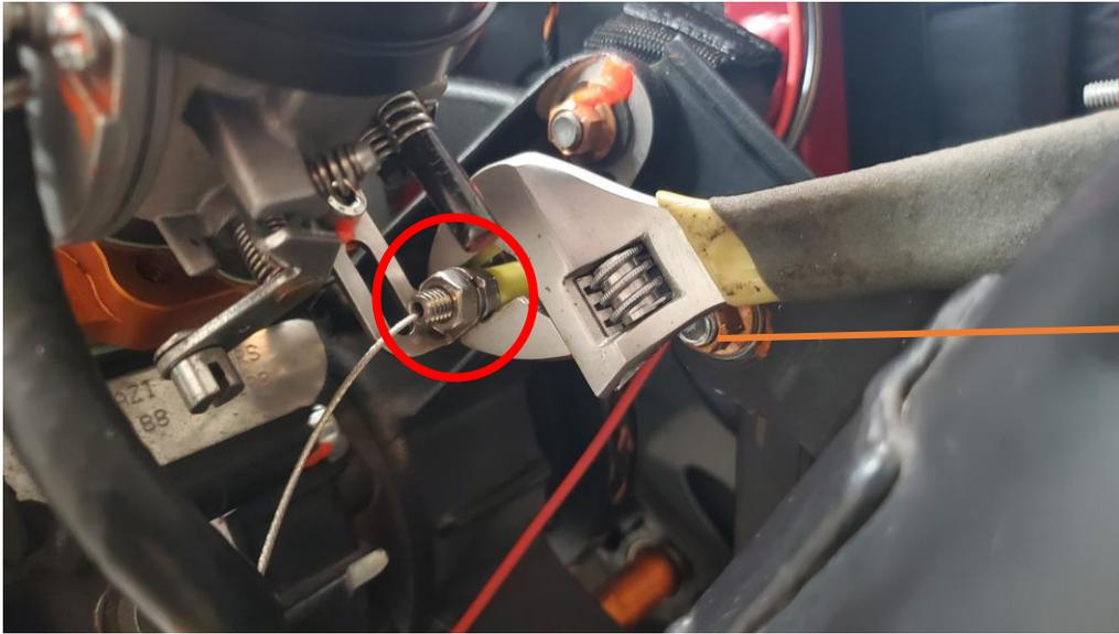
Using adjustable or 10mm wrench, grab onto rear hex nut.
