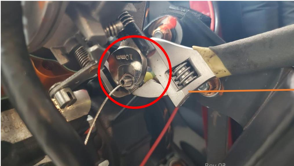
Use a second adjustable or 10mm wrench to lock down the two nuts over the barrel
