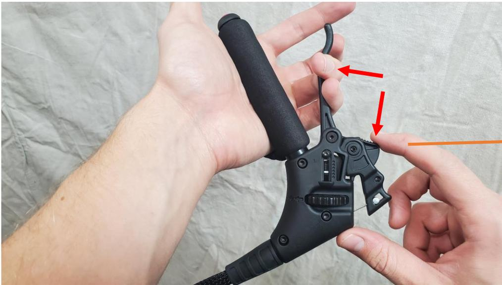
While in flight, keep pressure on the throttle lever and press down on the throttle lock as shown.
