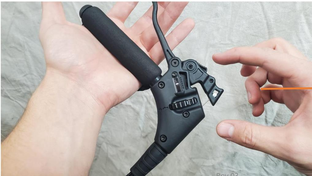
The cruise control can now be set, adjusted and disengaged easily by the pilot
