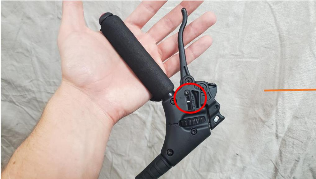
The throttle is back in manual control but the internal catch will remain in the last used position.
