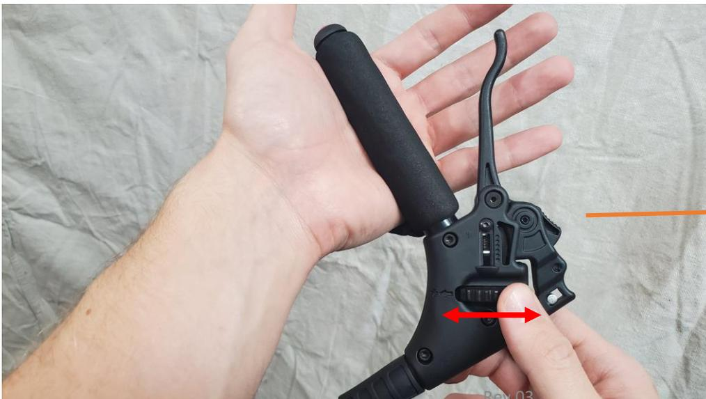
The engine should be running at low RPM based on the pre-set from earlier. Use the adjustment wheel to increase/decrease engine power until a desired cruise level is met.
