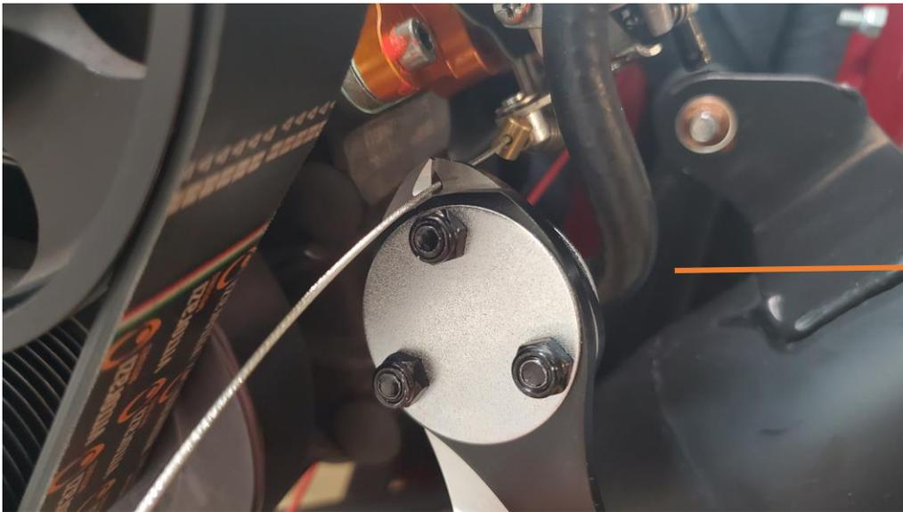
Leave enough room that the throttle can be removed in the future but not too much that the remaining tail will contact the prop.
