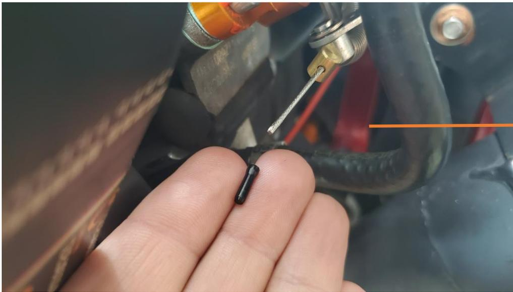
The end of the cable will be prone to fraying
