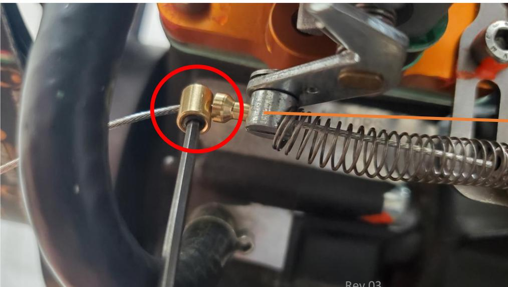
Using 2mm hex drive, tighten the set screw in the locking barrel
