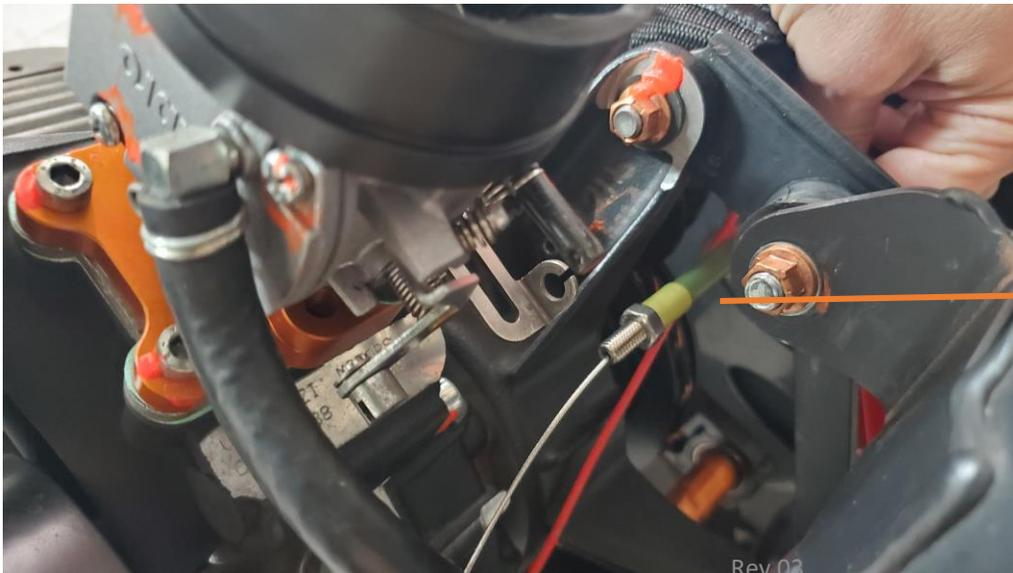
Feed cable through paramotor frame.
