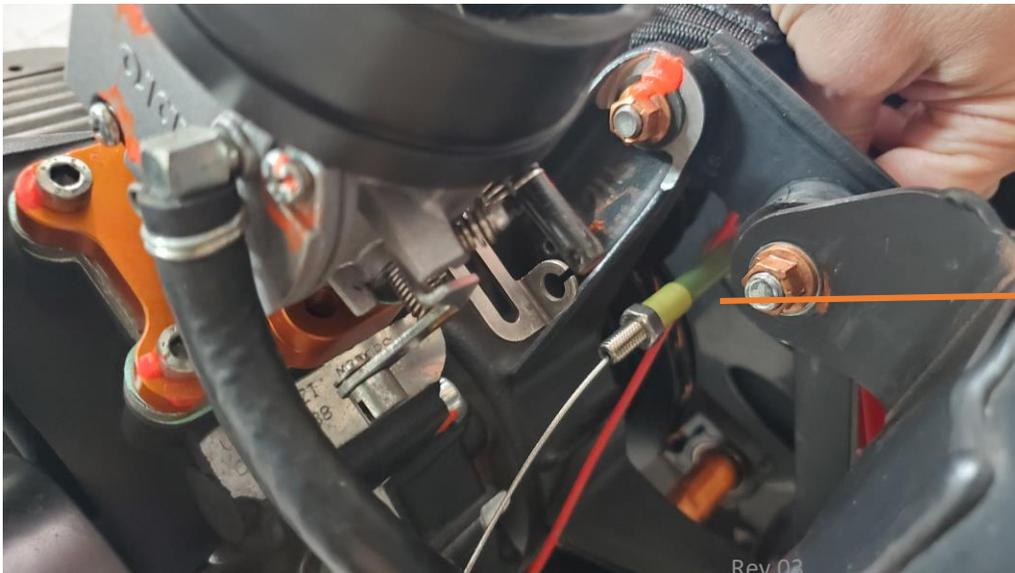
Feed cable through paramotor frame.
