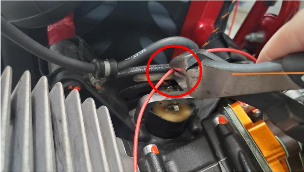
Feed the kill switch wire around the motor as desired and cut the wire to length.
