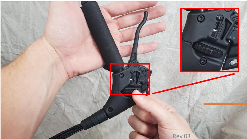
Continue to turn the wheel until the white notch is at or below the third dot on the side housing.
