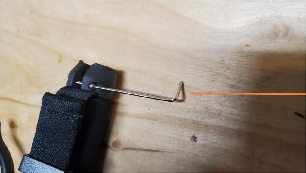
Tighten screw to lock the grip in place
