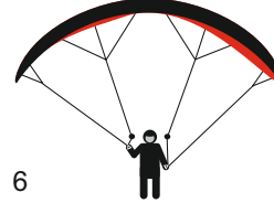
4 Extreme braking the central part - pull the inner lines down
