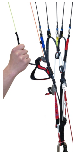
Steering with the TCT+ steering handle extensions (accelerated mode)
