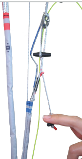
Closing the trimmer: pull the lower black bar down to the desired value.
