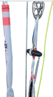
Trimmer in neutral position: pull the trimmer until the points on the line are visible on both sides of the black bar.
